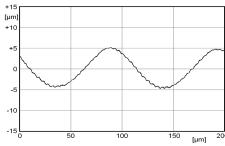
Stylus measured profile of a sinus standard (period 100 µm, PV 9 µm). Due to the manufacturing process of diamond turning, the sinus shape is overlapped by small profile amplitudes in the sub-µm range with partly large surface slopes.
