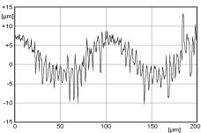
Optical measured profile of the same standard using a poor sensor design. The interaction light – surface which was not taken into account with due care results in false amplification of the profile amplitudes of several µm.
