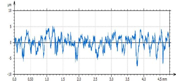
Calibration standard: **Rugo N7A (grinded)**
